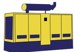
Running **below 30%** leads to significant increases in emissions per kWh (unit of electrical energy) used
